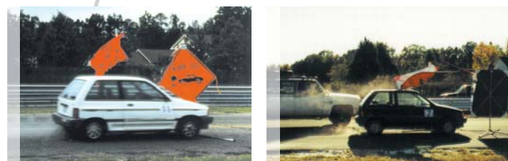
All KSI sign stands are NCHRP 350 Crash Tested and Approved with signs from 30" x 30" to 60" x 60", with or without flags and/or ballast
