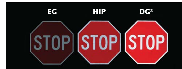
Nighttime comparison of Engineer Grade (Type I), High Intensity Prismatic (Type III/IV) and DG 3 (Type XI) Reflective Sheeting.
