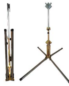
SS548E Full-size stand with two stage dual spring action base, kick release steel legs and an extended mast enabling a 21" and 5 ft. mounting height. Supports roll-up and rigid signs.
