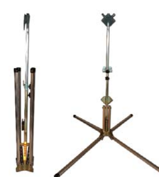
SS548AE Full-size stand with two stage dual spring action base with extended mast enabling a 21" & 5 ft. mounting height; kick release aluminum legs. Supports roll-up and rigid signs.
